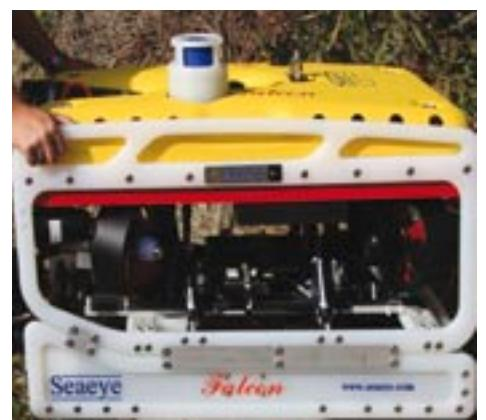
*uKwabelana* is equipped with a Seaeye Falcon remotely operated vehicle.
