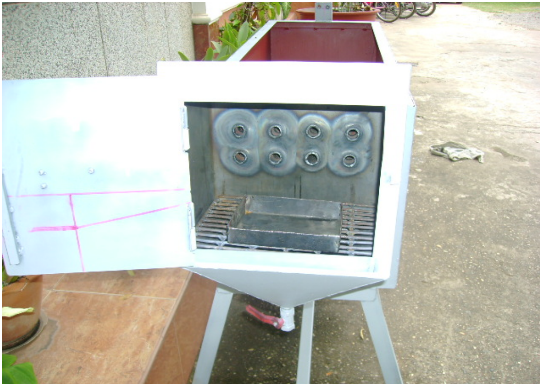
Photograph of Condenser Tubes Inside Stationary Retort
