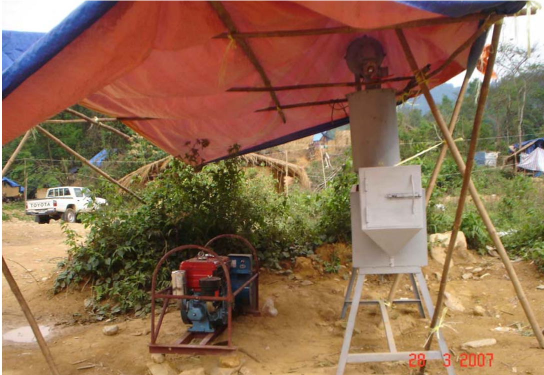
Photo of Stationary Community Retort Installed in New Mining Area near Nakadok Village
