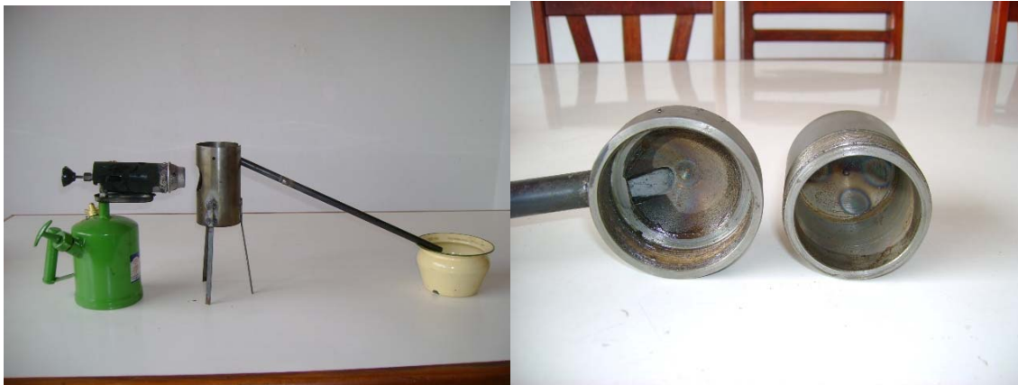
Photos of lathed retort in burning pipe produced in Vientiane with Chinese gasoline burner
