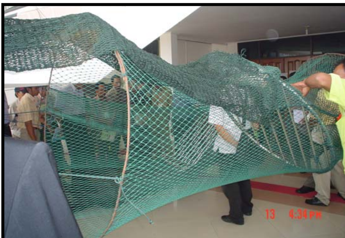
In-land practices: TED installation (net cutting, mesh counting, float attaching, etc)
