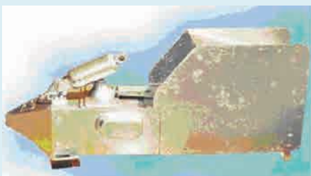
A basic Continuous Plankton Recorder. CPR technologies have changed very little in 40 years.
