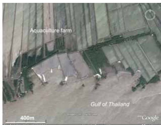
Figure 6: with kind support of Google Earth™ mapping service Satellite image of coastal erosion of the Chao Phraya delta near the river mouth. Mangrove collapse at the ocean front has led to a landward shoreline shift to beyond the aquaculture ponds. Approximate location is shown in Figure 2 (after Google Earth).
