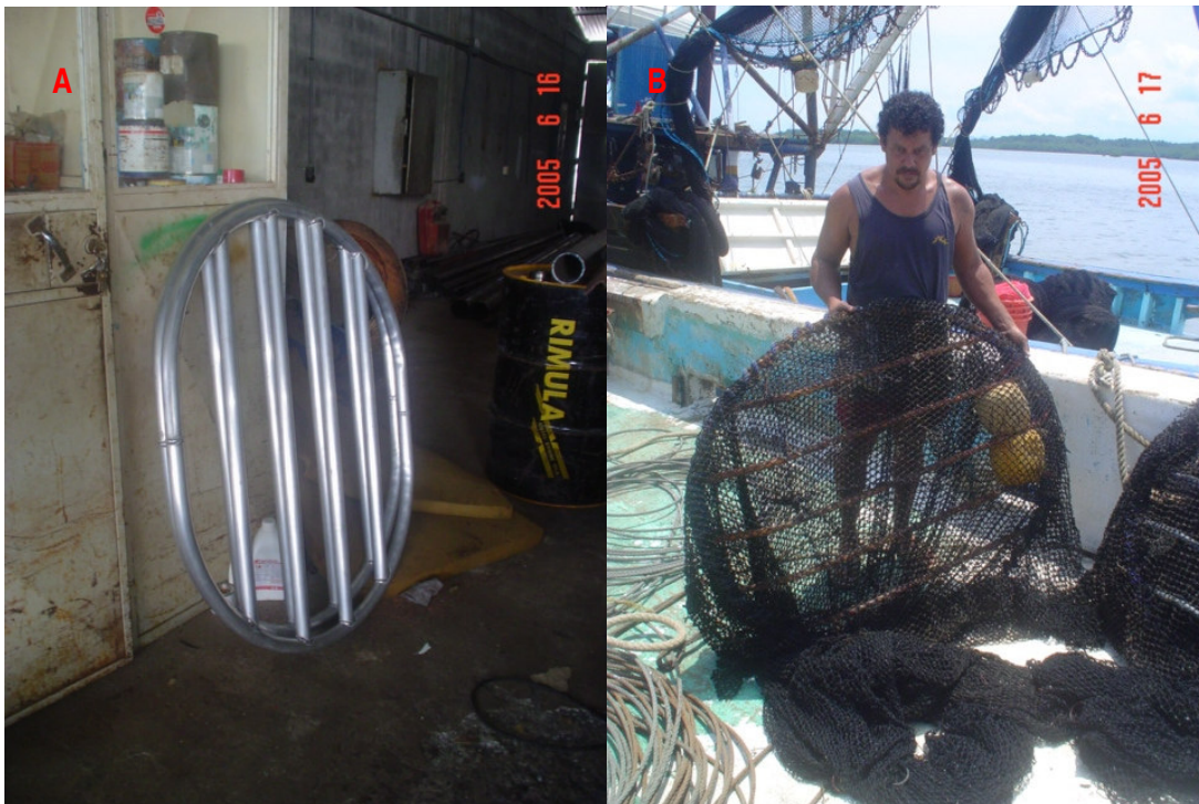
Figure 8. Photographs of the kinds of TEDs used in Costa Rica . A) Tico TED of inches and B) super shutter.
