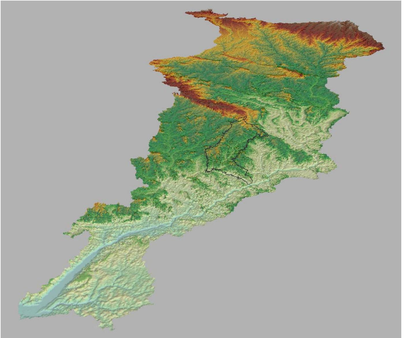
**Figure 14.** Perspective view of the Tapajós DEM, showing the limits of the Crepori basin in black (vertical exaggeration factor: 30x).
