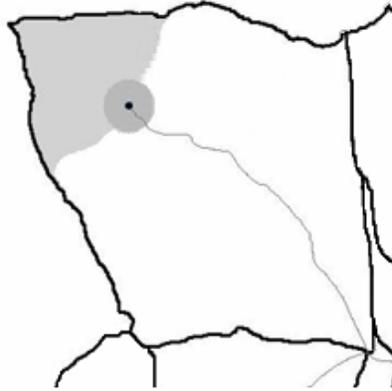
**Figure 5.** A 50m-buffer (dark gray) around a spring, overlaid on its drainage area (gray), compose the area to be protected.
