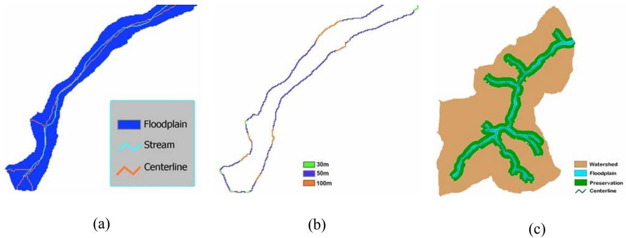
**Figure 6.** (a) Comparison between the original stream location and the centerline derived for its floodplain, (b) buffer's width as a function of the floodplain's width, (c) outline of the riparian zones to be protected bordering the floodplains.
