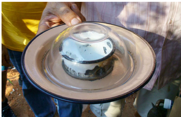
Gold like this contains residual mercury and should be burned again inside a fumehood
