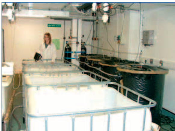
Figure 1: EPOCA investigates ocean acidification using a wide range of techniques: natural CO 2 vents, as well as laboratory and mesocosm experiments. The photograph illustrates the set-up designed at the Plymouth Marine Laboratory that is used to study North Atlantic and Arctic organisms. (Photo: S. Widdicombe, Plymouth Marine Laboratory)
