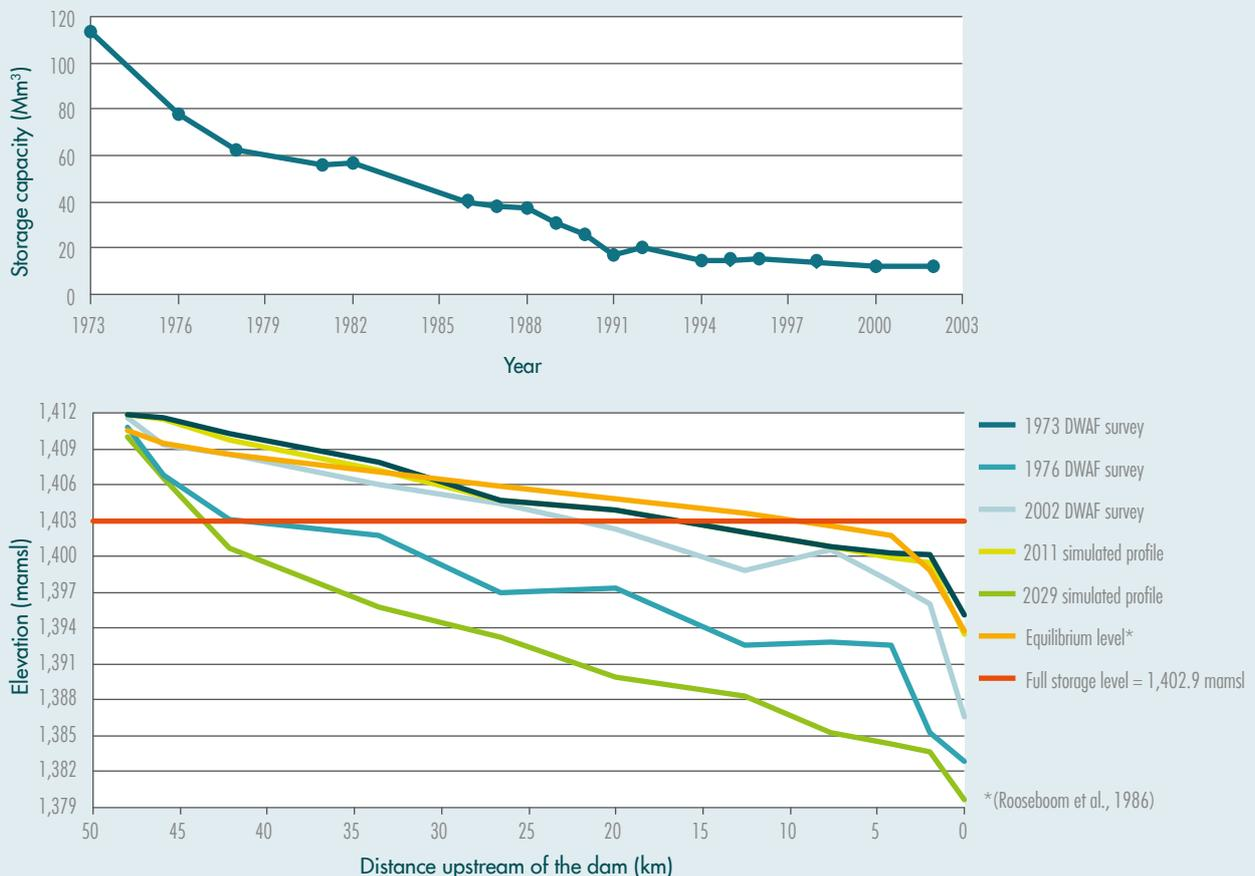
Figure 16: Storage capacity lost at Welbedacht Dam (top) and historical longitudinal bed profiles (bottom)
