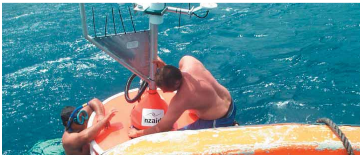
Deployment of a Sound Ocean Systems Inc water quality monitoring buoy in Manihiki Lagoon funded by bilateral NZAID to the Cooks Islands and installed and monitored by the SOPAC OI programme.
