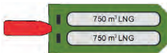
Figure 33: Sketch of a 1 500 m 3 LNG barge connected to a harbour tug
