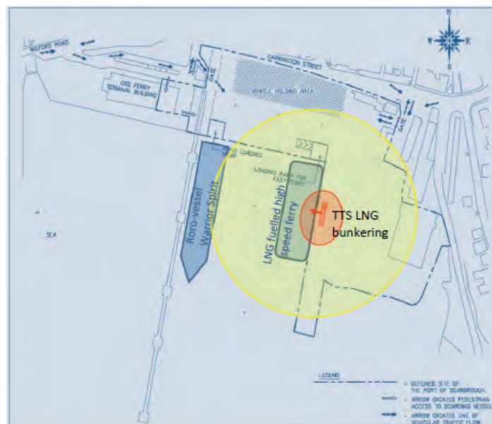
Figure 43: An indicative 25 m safety zone surrounding a TTS LNG bunkering arrangement in Scarborough ferry terminal
