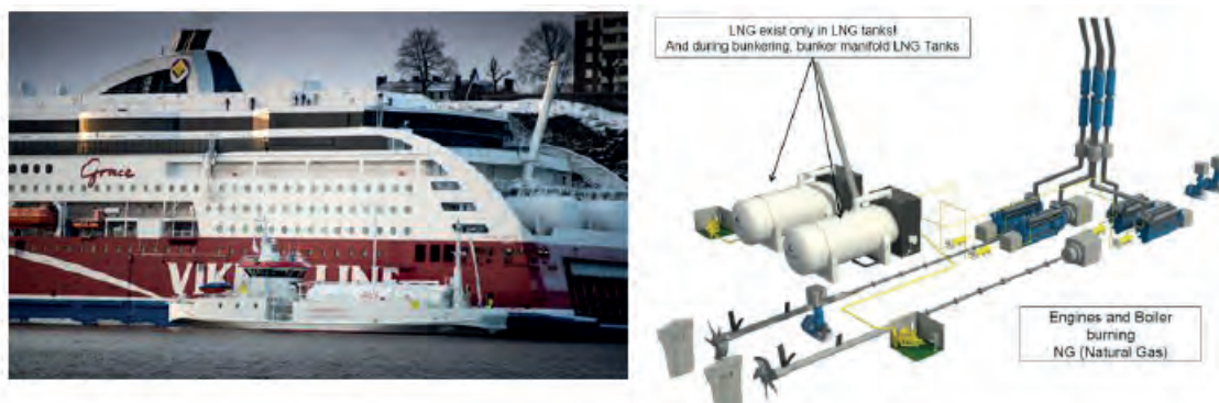
Figure 7: VIKING GRACE and the LNG bunker barge moored alongside at the ferry's bunker station. Engine and propulsion arrangement (Granberg, 2013)
