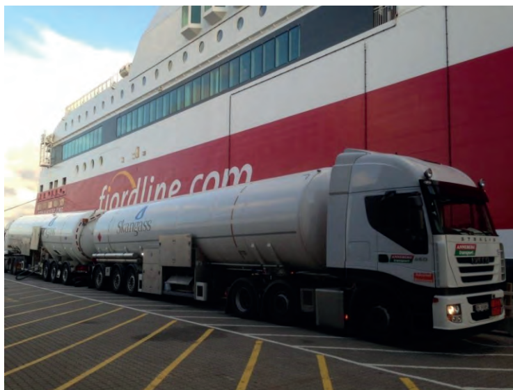
Figure 21: Truck to ship bunkering (TTS) of LNG from two trailers in parallel (Photograph reproduced courtesy of Skangass AS)
