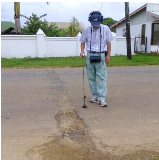
Figure 13 Leak detection in Neiafu
