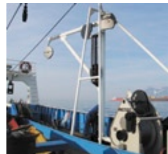
A new winch and davit were installed on the Tombwa's port side to facilitate the towing of small plankton nets
