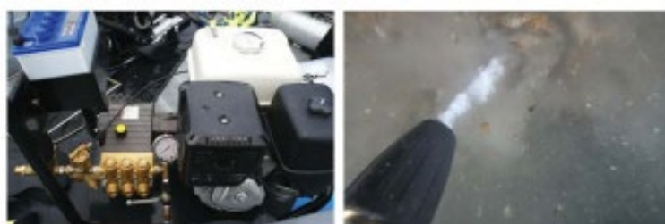
Underwater jet machine and its use in jellyfish polyp removal.
