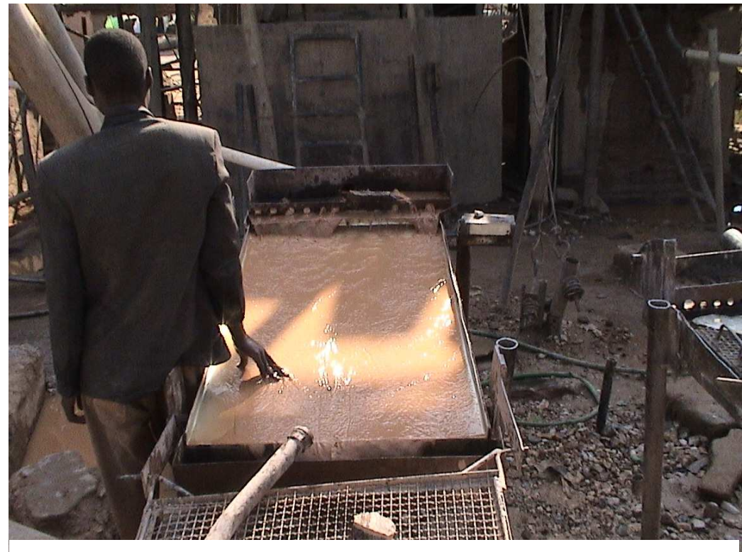
The whole ore is amalgamated using a Copper plate
