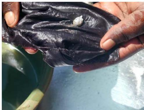
F: Amalgam after squeezing to remove unused mercury
