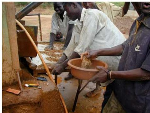
D: Copper plate cleaning by hand with sand and cyanide tablets
