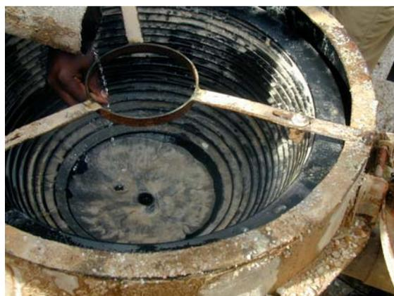
b) Remaining amalgam droplets in the riffles
