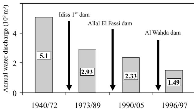
**Figure 2.** Reductions in the Sebou water discharge at Mechra Bel Ksiri (downstream measuring station) following the construction of three dams between 1972 and 1996 (Haida, 2000).
