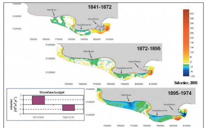
**Figure 3. Sedimentary losses (1895 to 1974/88) on the upper shoreface (0-20 m). Bathymetric comparison and shore face budget.**
