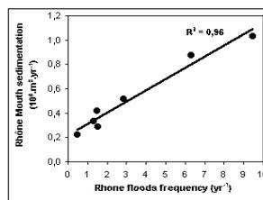
**Figure 2. Slowing down in sedimentary input at the Rhône mouth ( $\times 10^6$  m<sup>3</sup> yr<sup>-1</sup>) according with reduction of the frequency of the major floods since 1841.**
