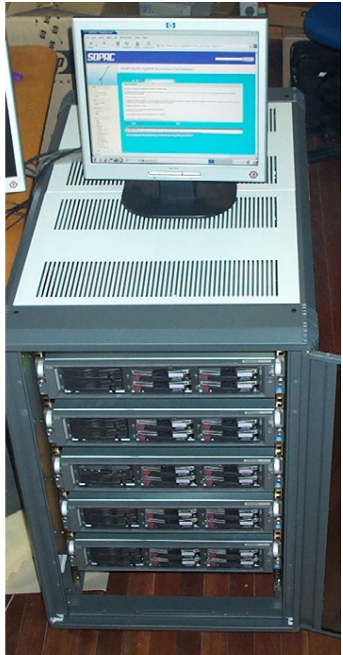
Example of a typical "Map Server" configuration used to establish National Information Centres within PICs. The Map Servers are set up at SOPAC prior to shipping and is sufficient to run the ICT functions of the national government of a small island state.
