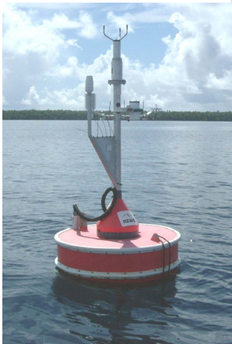
Monitoring buoy, Manihiki Lagoon. Part of initiatives to monitor physical oceanographic parameters in the lagoon to determine impacts on pearl fisheries.
