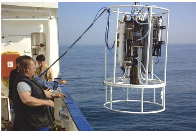
*Figure 1: A cast is being prepared to take water samples and to make measurements of optical properties of phytoplankton and suspended matter in the North Sea.*
