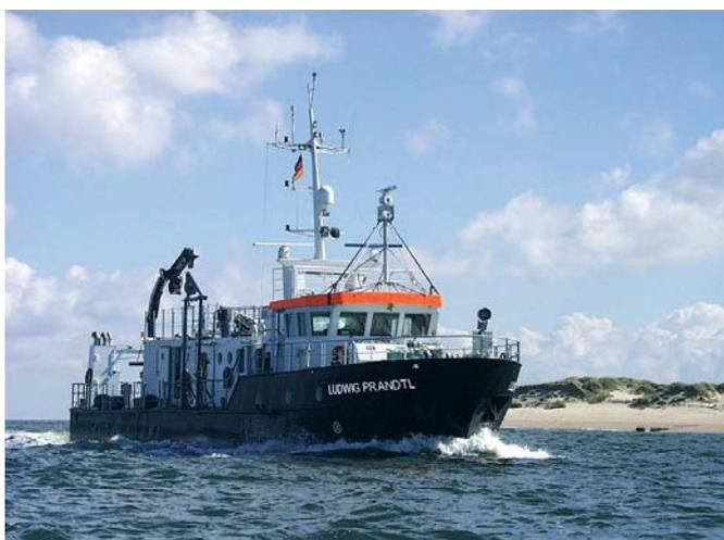
*The GKSS research vessel Ludwig Prandtl was designed specifically for use in shallow coastal waters.*
