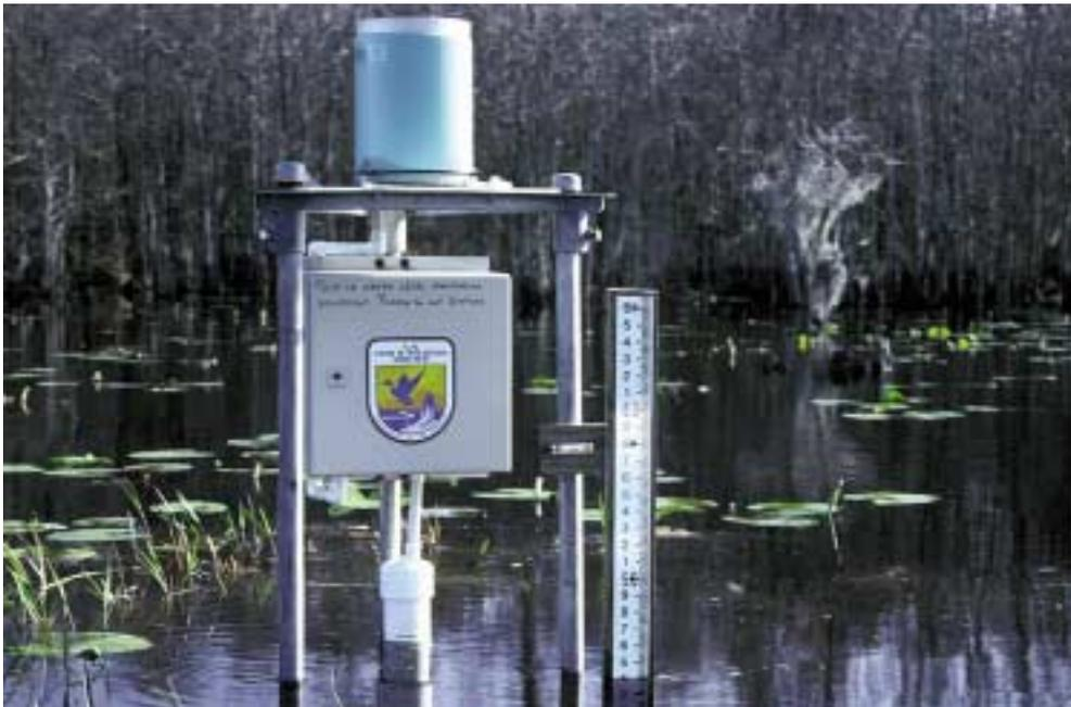
Water level monitoring is an essential element of environmental flow management.
