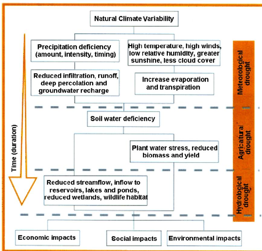
Figure 1.3 - Natural climate variability and hydrological cycle.
