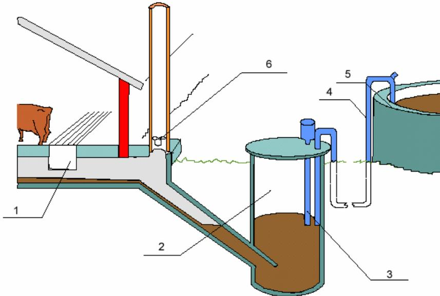
**Figure 10.3 - Slurry removal system: 1 - slurry channel, 2 - pit for pumping over; 3 - pump; 4 - rising pipe of slurry, 5 - slurry reservoir, 6 - ventilator** (after *Code of Good agriculture Practices for Lithuania*)
