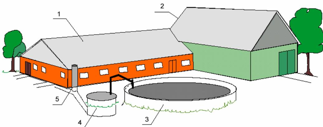
**Figure 10.2 - Non littered barn with feed storage and manure storage: 1 - barn; 2 - feed storage; 3 - slurry reservoir; 4 - pit for pumping over of slurry; 5 - ventilation pipe (after Code of Good agriculture Practices for Lithuania)**
