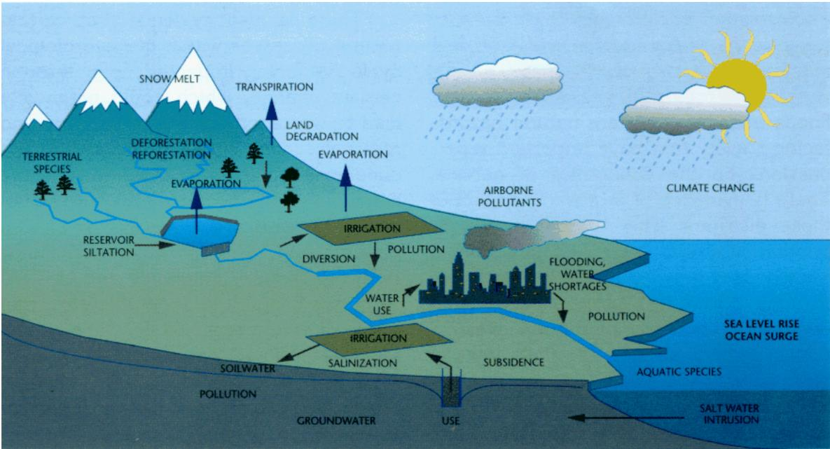
Figure 1.1 - Hydrological cycle with some aspects of the human – induced stresses.
